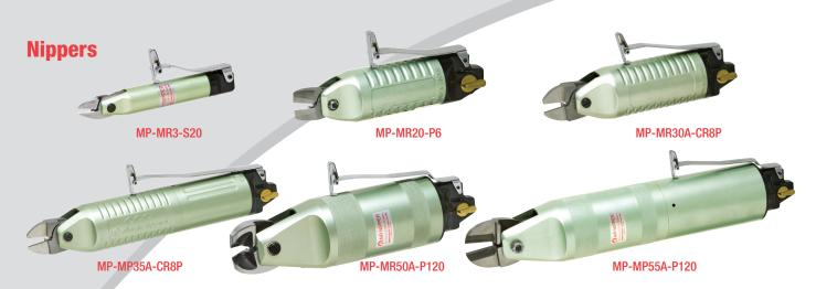
Powerful, lightweight nippers designed for a variety of applications, including pressing, riveting, bending and plate cutting. Ideal for cutting copper wire and soft materials. Larger units are perfect for cutting plastics, stainless steel and piano wire. Optional blades available.
